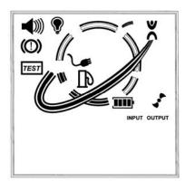
The display shows the UPS in BYPASS MODE. The solid line is connected from the Input to Load. Another solid line is connected from the Input to Battery in charging. The Fan is in low speed; Line and Charger icons are illuminated.
